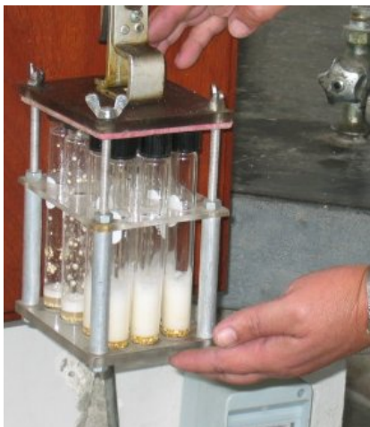
The more saponin quinoa has, the more foam it makes when shaken in a test tube.
